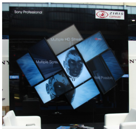
Sony Ziris Canvas demonstration wall designed to be erected in 4 hours and fits into 3 flight cases including all screens and PS3's
