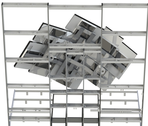
Sony Ziris Canvas demonstration wall designed to be erected in 4 hours and fits into 3 flight cases including all screens and PS3's
